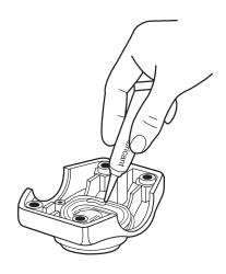
7. Install your Nature<sup>2®</sup> Express on schedule 40 PVC pipe only. Failure to heed this warning can result in equipment failure. Position the clamp assembly on the pipe, with the arrow pointing in the direction of the flow of water and hand tighten the nuts and bolts. Tighten nuts an additional 1/4 turn using a wrench or socket. Do not over-tighten.
