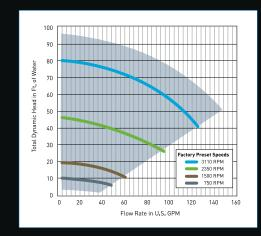
NOTE: The chart to the left demonstrates performance rates at factory preset speeds of 750 RPM, 1500 RPM, 2350 RPM and 3110 RPM. However, flow rates can also be custom programmed between the ranges of 400 RPM and 3450 RPM as indicated by the blue tint.
